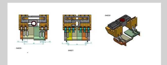
Special double-needle sewing foot - two to six-part waistband production
