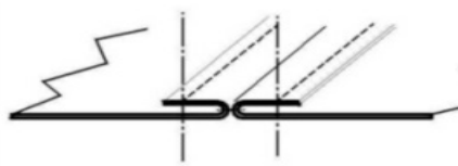
Seam diagram, bust cross seam with and without tape
