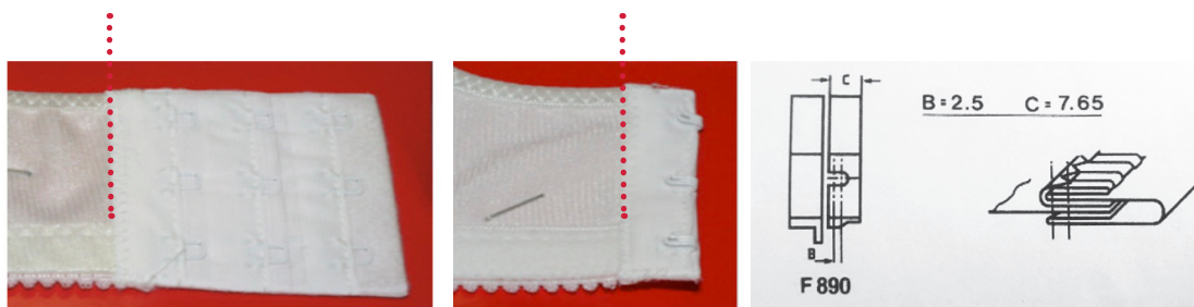
Hook tape sample Zigzag seam with exact edge guide for brassiere closure
