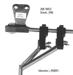
Swing-up edge stop with two stops to right of needle
