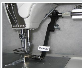
Pneumatic swing-up multi-position edge stop up to four edge distances can be retrieved.
