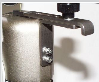
Fabric edge stop to right of needle on a post-bed sewing machine
