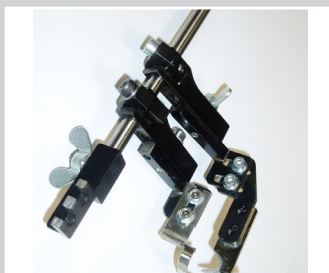
Two fabric edge stops swiveling up to right of needle
