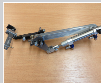
Pneumatic swing-up fabric edge stop to right of needle with cylinder for two edge distances.
