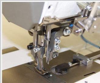
Punching knives on a flatbed/ drop feed/sewing machine with pneumatic edge guide
