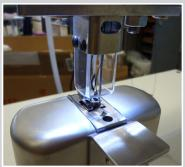
Stick shift bellows sewing devices for turnover seam
