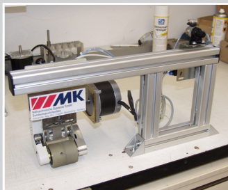
Puller, two-piece, 54 mm with step motor stationary behind machine
