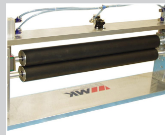
External puller, with powered trans- port rollers above and below. Drive motor acc. to choice, roller widths from 35 to 600 mm. With or without motor control.
