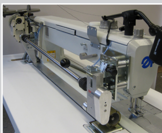
Puller, one-piece, with powered transport rollers above and below roller diameter 54 mm
