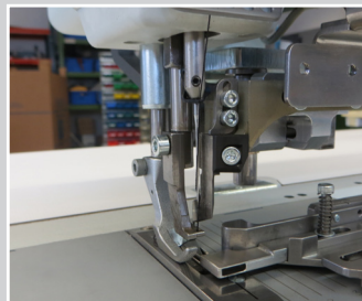
Piping guide for glued leather piping
