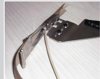
Piping guide for open leather piping with pin-tuck
