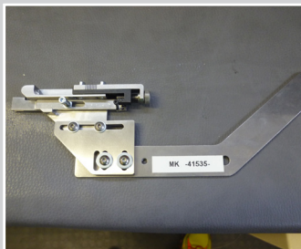
Piping guide for glued leather piping
