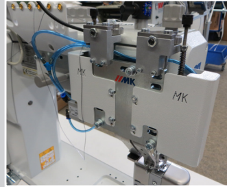
Seam center guide and plow guide with reproducible precision height adjustment on a post bed machine
