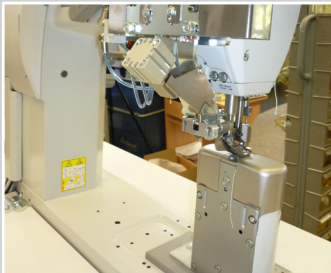
Seam center guide and plow guide with forward/back adjustment on a post bed machine
