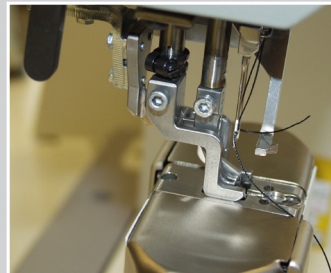
Seam center guide and plow guide extra high at rear on a post bed machine
