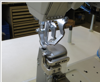
Fell seam guide, 2-part right with inclined roller with pneumatic guide from below
