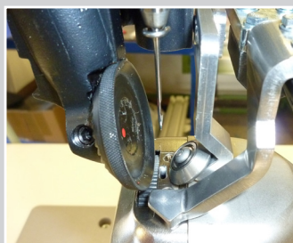
Fell seam guide, 2-part right with inclined roller
