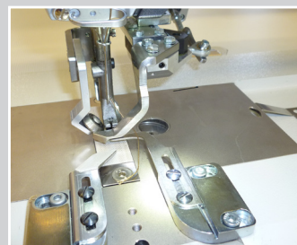
Fell seam guide, 2-part left with inclined roller with seam folder left and right on a flatbed machine
