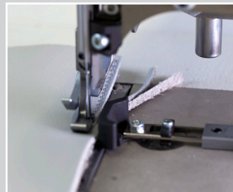
Counter knife normal version, on a flatbed/wheel feed/ sewing machine with pneumatic edge stop
