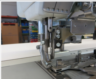
Counter knife on a flatbed/ drop feed/sewing machine, hook on right, with integrated Piping Guide
