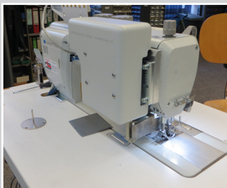
Counter knife on a flatbed/ drop feed/sewing machine, hook on right, short thread trimmer
