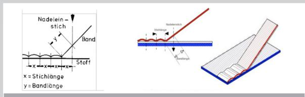
Tapes and lace fed in from above are loosely sewn on through penetration of the sewing needle in the inclined guide channel.
