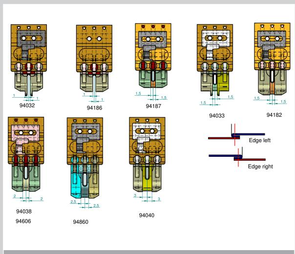
Special single-needle sewing foot - sewing left and right side seam, three-part Fully automatic alignment of the stop sole by the material
