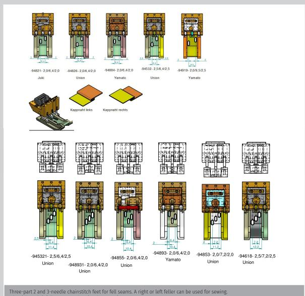
Three-part 2 and 3-needle chainstitch feet for fell seams. A right or left feller can be used for sewing The right or left fell seam can therefore be sewn from top to bottom
