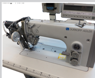
Tape feed with cutter on a lock-stitch machine
