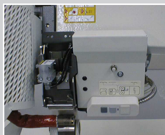
Tape feed with cutter on a hot air sealing machine
