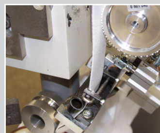
Tape feed with cutter and length metering device for a hot wedge sealing machine
