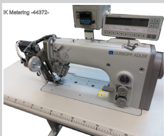
Small tape cutter on a single needle machine. With length metering device for sewing spacing stripes on blankets
