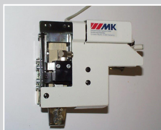
Small tape cutter on a Strobel blind stitch machine
