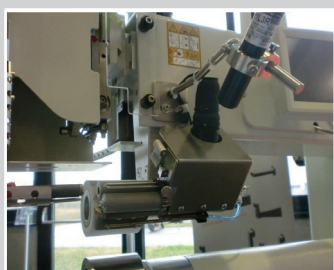
Strong tape cutter on a hot air sealing machine, cutting width 55 mm
