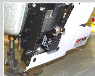
Small tape cutter on a zigzag machine
