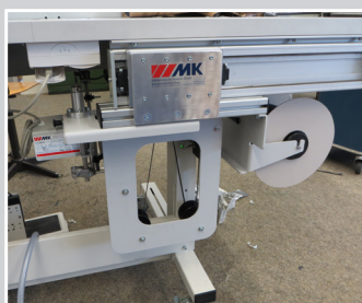
Tape roll holder with lateral extension, with integrated tape monitor and tape dispenser for fitting under the tabletop
